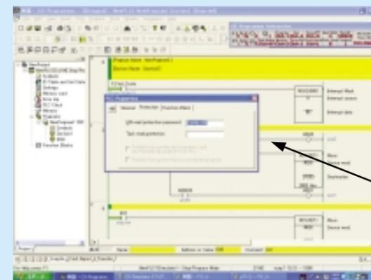
Important programs can be protected by setting a password from the CX-Programmer (with the PLC online).
